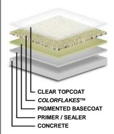
For best results, 10-15 mils of clear top-coating is recommended to fully encapsulate *ColorFlakes*<sup>TM</sup> and provide a durable wearing surface.
